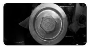
The check plug is located at the top center of the inside case of each transaxle. The transaxle can be filled with oil by removing these check plugs from both transaxles and pouring the oil in the hydro overflow tank, located behind the seat. Oil will begin to run out of the check plug holes when the transaxles are full. Use only 20w50 motor oil in the hydro system.
