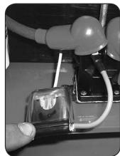
Always check the condition of the wiring harness ground cable. The ground is located just inside of the right side fuel tank on most models. Ensure that the ground is connected, clean, and tight. On some models, this wire may be connected to the negative side of the battery.
