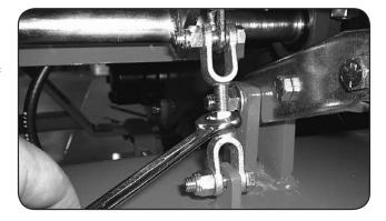
The large turn buckles on the front of the deck only affect the pitch of the deck or the level from front to back.
