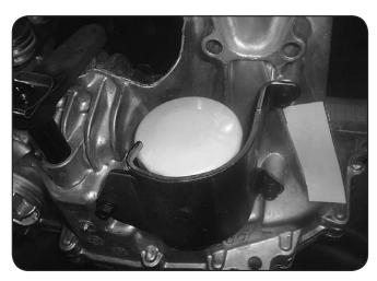
Shown right is the CZT transaxle. The large cap on the lower left is the filter housing cap.
