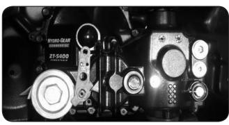
Filter housing cap. (do not over tighten)
