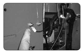
Check the condition and connection of the relays located under the seat. Ensure that they are clean and connected. Make sure that wire terminal ends have not been pushed out of the relay block.
