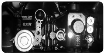
5400 filter housing cap. (do not over tighten)
