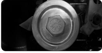
The check plug is located at the top center of the inside case of each transaxle (outlaw transaxles have this plug on the top). The transaxle can be filled with oil by removing these check plugs from both transaxles and pouring the oil in the hydro overflow tank, located behind the seat. Oil will begin to run out of the check plug holes when the transaxles are full. Use only 20w50 motor oil in the hydro system.
