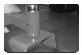
There is one grease fitting on each of the actuator bar pillow blocks located under the fuel tanks. Grease twice a season.
