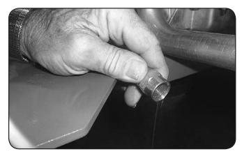
The fuel filter is located in the fuel line about 12" from the carburetor on the side of the engine. Note the direction of flow on the side of the filter. Replace once a year.
