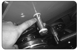
The deck belt tensioner is located at the rear of the deck and has a grease fitting on its pivot point. Grease at every engine oil change.
