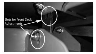
The deck spring tension is critical. If the tension is too high, premature failure of the deck belt and blade spindles can occur. If the tension is too low, the belt can 'jump off' or slip on the pulleys. This results in reduced cut quality and early belt failure. Spring tension adjustments can be made by sliding the bolt shown above forward or backward in the slot of the deck Belt tension should be set between 60-65 lbs. with the deck at its lowest setting.
