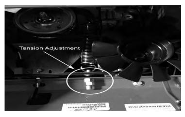
The tension should be adjusted so that there is between 50 to 55 lbs. of tension on the belt. This can be checked with a belt tension gauge as shown to the right.
