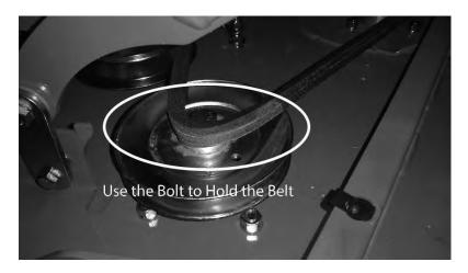
(5) Check to make sure the belt is on all the pulleys and matches the belt routing
