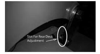
If deck adjustments are necessary, the deck hanger bolts have adjustable slots. These adjusters affect the overall height of the deck and the level from left to right.
