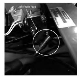
When adjusting the tracking on the mower, the length of the pushrods can be changed by screwing the swivel joint in or out on the ends of the rods. Shortening the overall length of the rod slows the pump down. Lengthening the rod will increase the speed of the pump.
