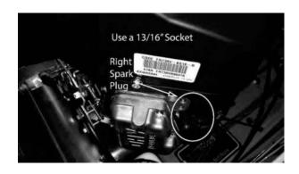
2. Check the gap on the spark plug to verify that it is 0.03" by using a feeler gauge.
