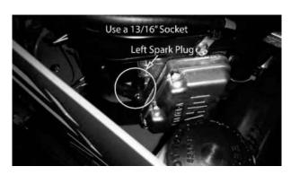
3. If the spark plug is worn, overheated, wet, or carbon fouled replace the spark plug.
