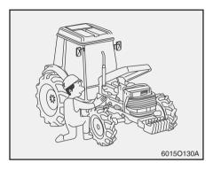
Stop and cool down the engine before fueling or lubricating;
