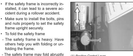
(1) Position Control Lever (A) Lowering (B) Lifting
