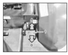
(1) Differential Lock Pedal (A) Release (B) Engage
