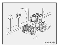
Avoid rapid starting, braking, turning, and excessive speed;
