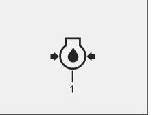
(1) Engine Oil Pressure Warning Lamp
