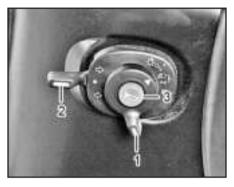
(1) Lamp Switch(2) Turn Signal Lamp Knob(3) Horn Button
