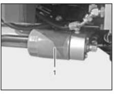
REPLACING TRANSMISSION FLUID FILTER
