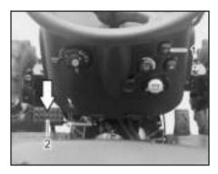
(1) Cruise Control Switch(2) Brake Pedal
