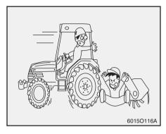
Put machine shut down sign if the machine is stopped on the road;
