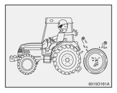
Turn off engine in a level area when leaving the tractor;
