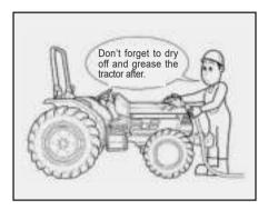
After work, clean the tractor. After cleaning, dry the moisture and supply grease into each grease nipple.
