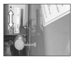
(1) Position Control Lever (A) Lowering (B) Lifting
