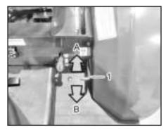
(1) Differential Lock Pedal(A) Release(B) Engage
