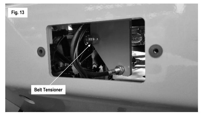
The pump belt tension should be set between 60-65 lbs. This should be measured with a belt tension gauge. Your dealer or service center will have a belt tension gauge or you can buy one (Part Number 041-9999-00).
