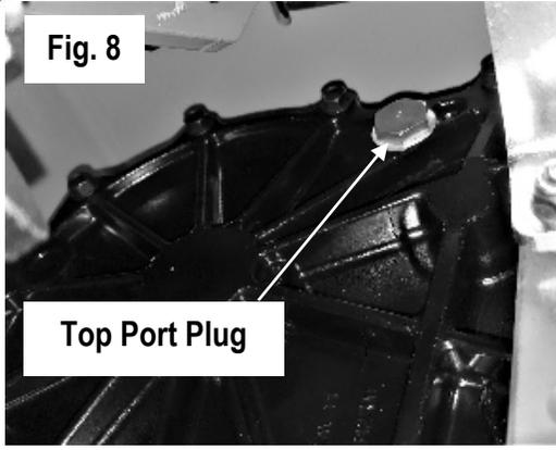
11. Install and torque the top port plugs to 180 in. lbs. (20.3 Nm).
